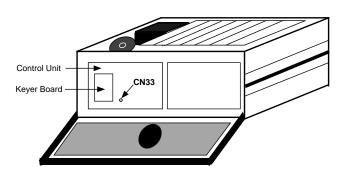
TS-950 with covers removed and front panel tilted down showing the Control Unit PC Board, including CN33, and the keyer "daughter" board.
