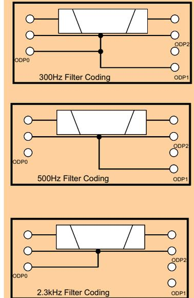
Figure 3. CW Filter Coding (Optional on the FT-817)
