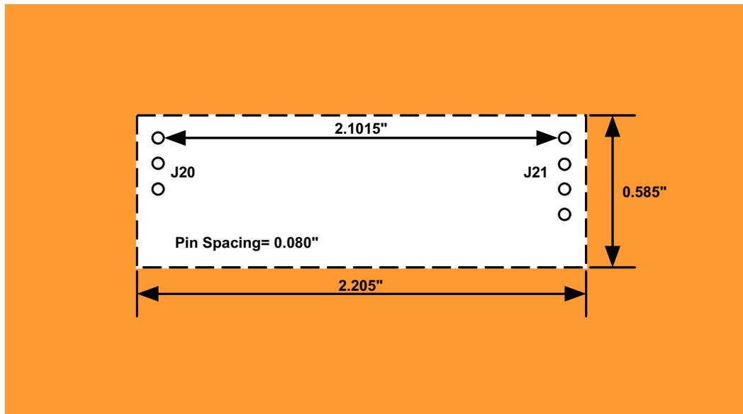
Figure 2. FT-817 main board layout showing reserved area and pin spacing for the accessory filter.
