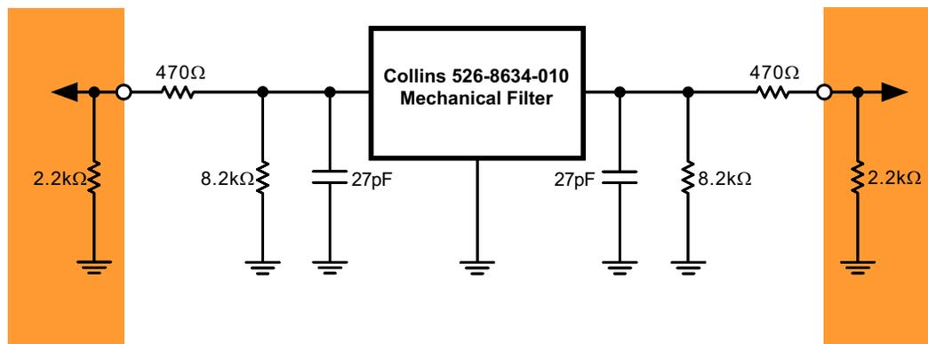
Figure 1. CW filter circuit schematic
