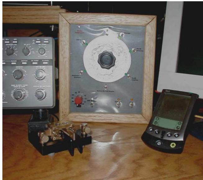
**Figure 1. The Operator Console and Display (for Station 4). Note the Azimuthal map inside the direction control.**
