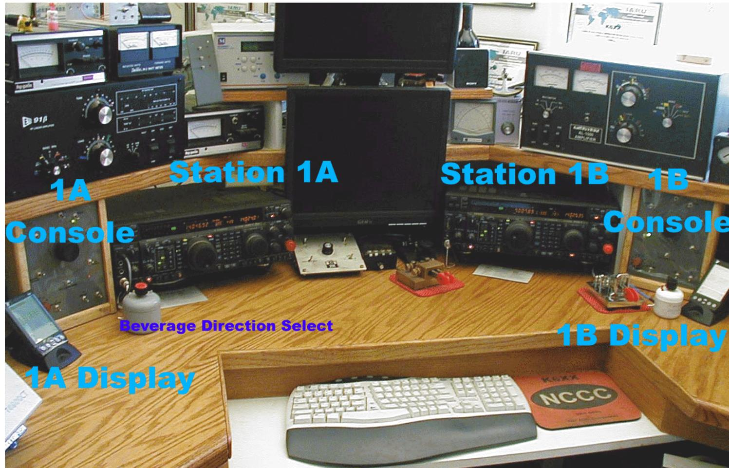
**Figure 5. K6XX S02R Station 1 showing the antenna select system operator interface.**
